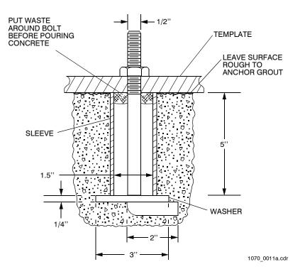
Figure 3-5. Typical Foundation Bolt Configuration
