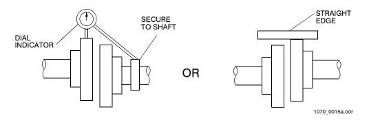
Figure 3-9. Checking for Parallel Coupling Misalignment
