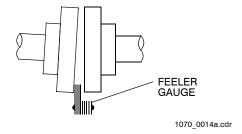
Figure 3-8. Checking for Angular Coupling Misalignment
