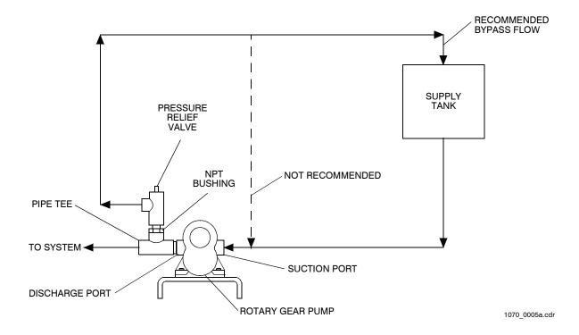
Figure 3-11. Pump By-pass Piping
