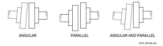
Figure 3-7. Types of Coupling Misalignment
