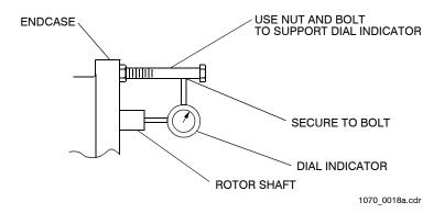
Figure 2-5. Rotor Clearance Adjustment
