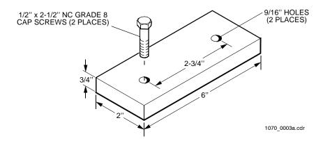
Figure 2-2. Timing-Gear Puller Fabrication Diagram
