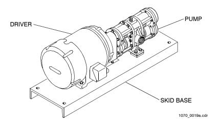
Figure 3-1. Typical Pump Skid
