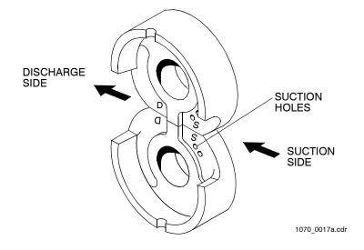
Figure 2-3. Liner Installation
