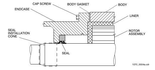
Figure 2-4. Single Lip Seal Installation
