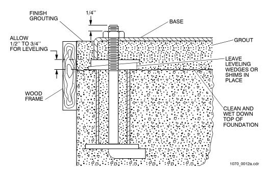
Figure 3-6. Leveling and Grouting Diagram
