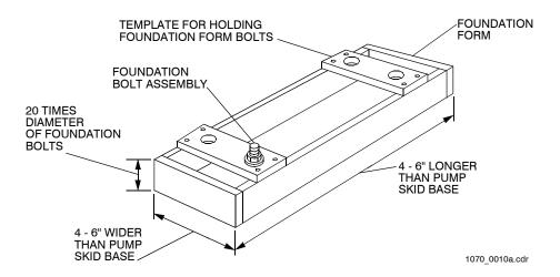
Figure 3-4. Typical Foundation Form
